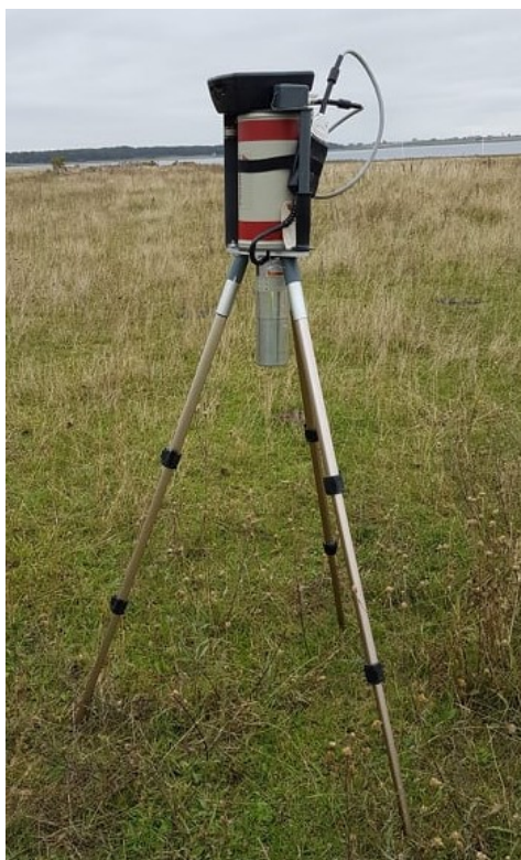
Figure 5: In situ gamma spectrometry at site 1 with a HPGe detector.
