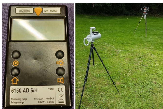
Figure 11: Handheld radiation protection unit (left) and scintillator probe on a tripod facing the HPGe detector(right).
