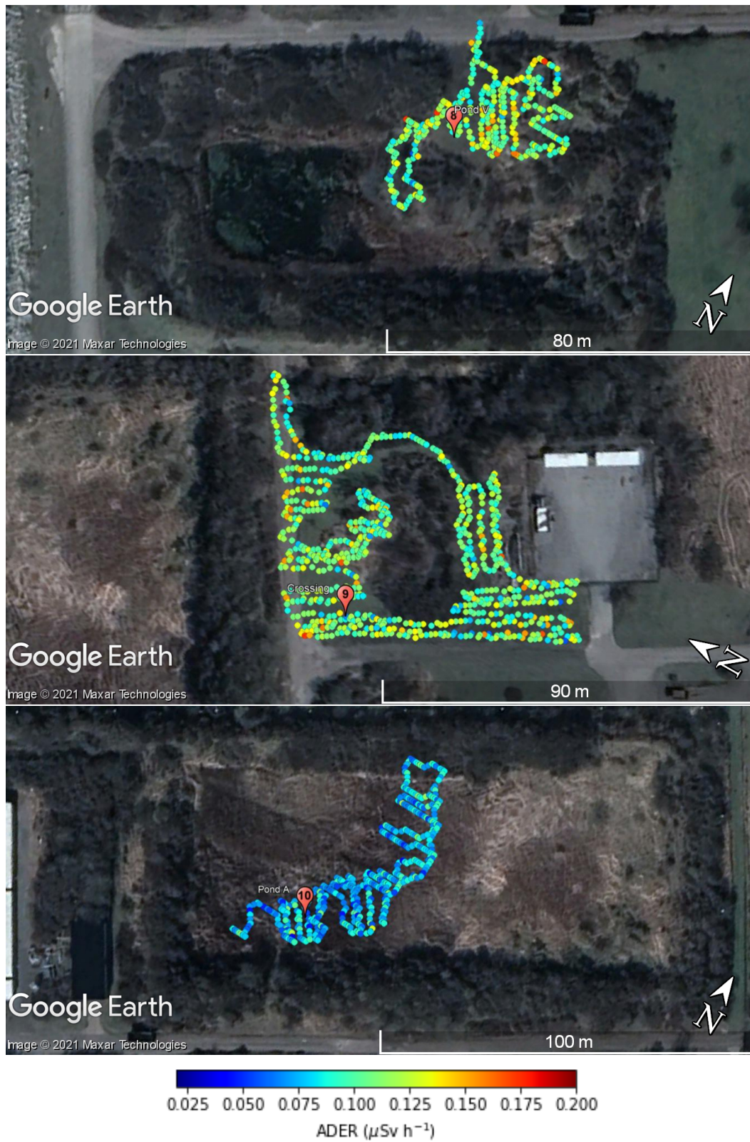
Figure 18: Mobile gamma spectrometry inside the fenced area (sites 8-10) covered with backpack measurements.
