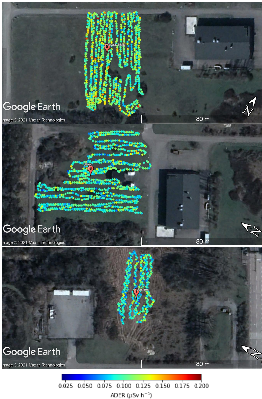
Figure 17: Mobile gamma spectrometry inside the fenced area (sites 5-7) covered with backpack measurements.
