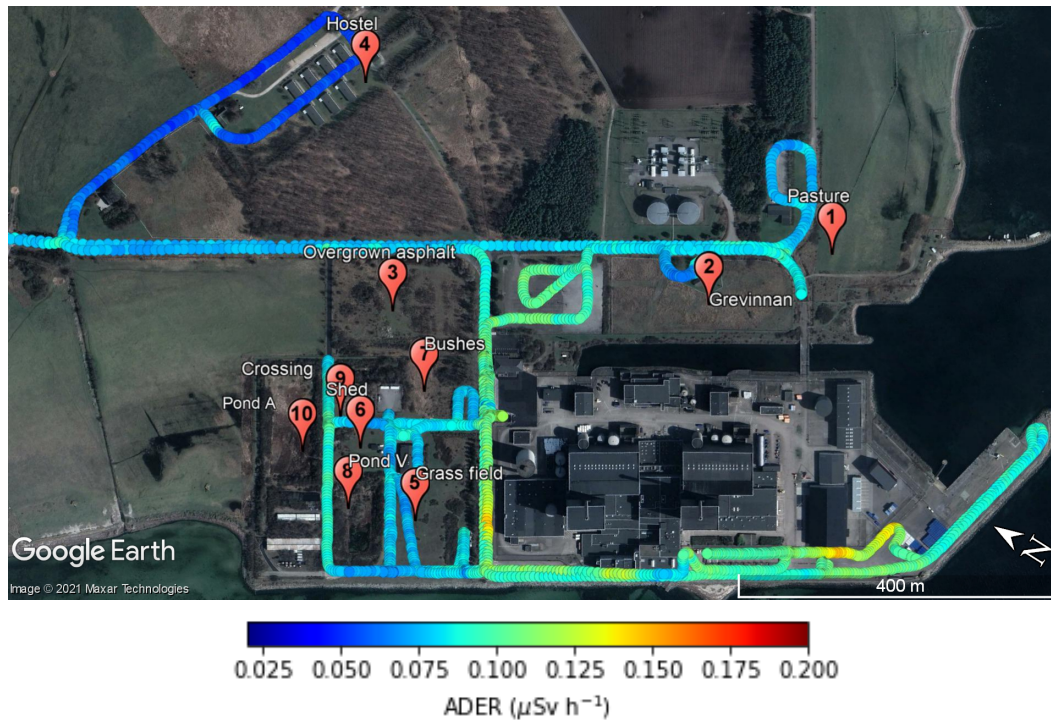
Figure 14: Car-borne mobile gamma spectrometry measurement with color coded ADER.
