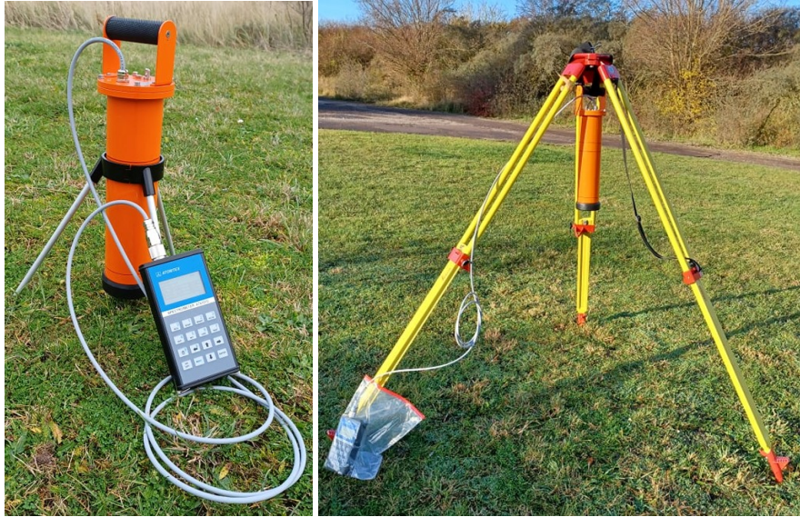
Figure 6: AT6101D in situ gamma spectrometry/ADER measurement 0.1 meter and 1 meter above ground at site 9.
