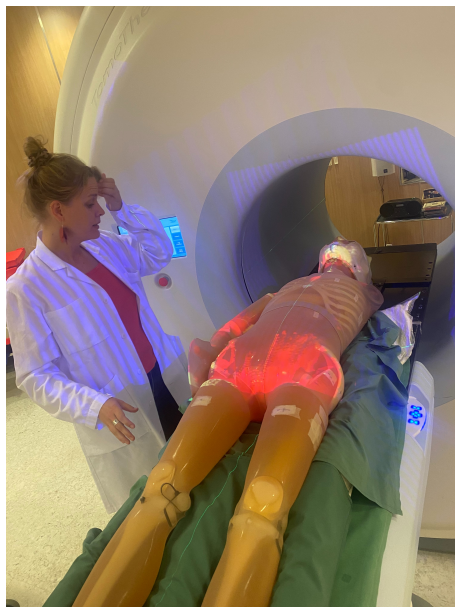
Figure 7: Whole body phantom (Kyoto Kagaku, Kyoto, Japan) positioned in a TMI immobilization at the Radixact positioned with OSS system.
