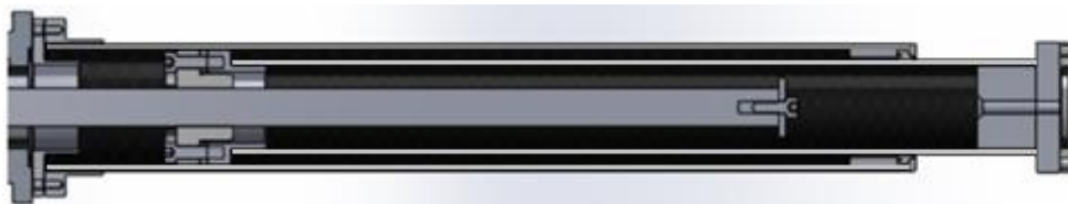
Figure 9: The second version of the actuator using a carbon tube as cover.
