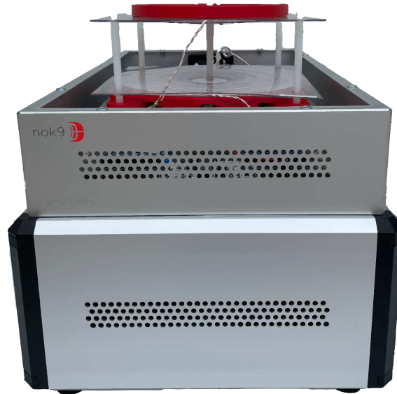
Figure 4.9: EVA III MDT with the main Tx, NFC Tx, NFC Rx, and main Rx coil mounted.
