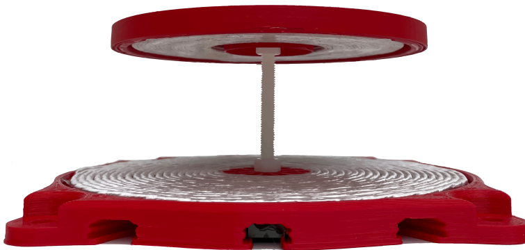
Figure 3.1: Main Tx coil (bottom) mated with the main Rx coil (top).
