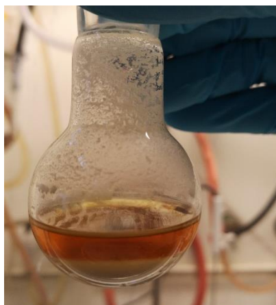
Figure 4.10 Polymer precipitated (bottom) in NMP and pyrrolidine solution (top).
