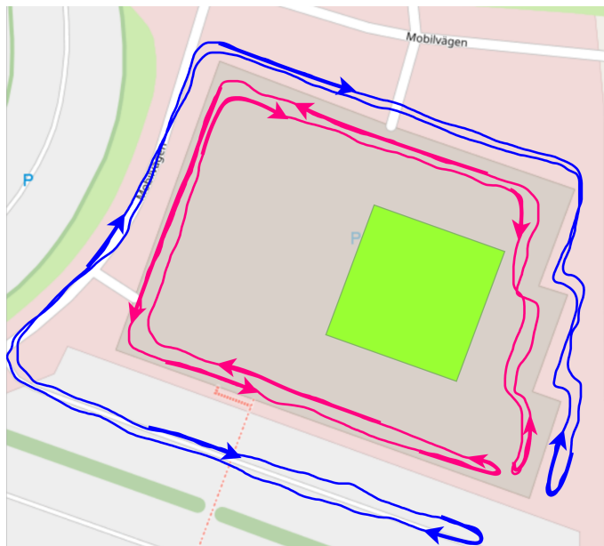
Figure 6.3 The collection plans for the three datasets: the blue path is the approximate NLoS predictable path, the purple path on the top of the garage is the approximate LoS pathway, and the vivid green geometry shows the approximate region for the dense-walk dataset.
