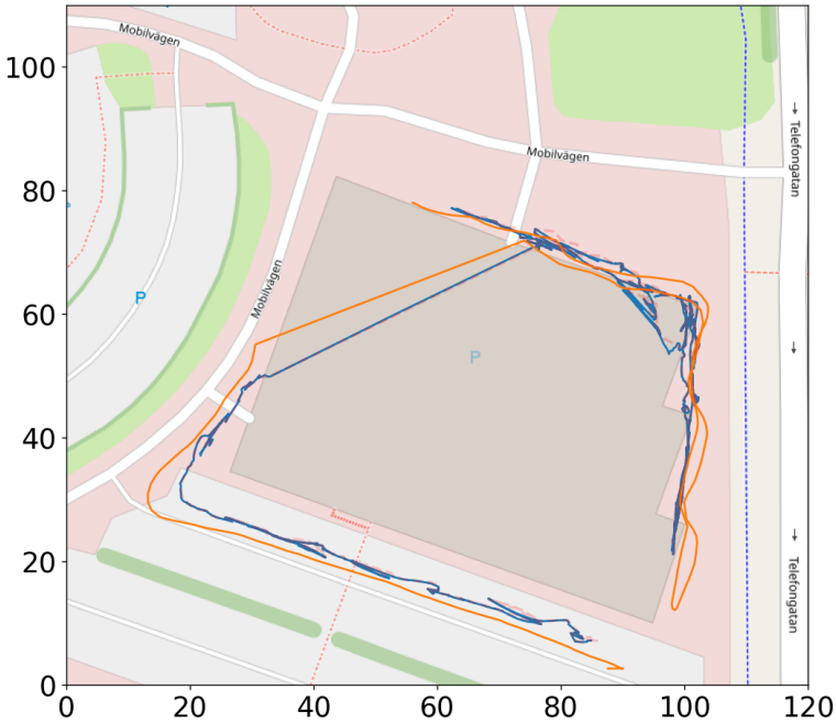
Figure 11.5 A part of the output of feeding the particle filter algorithm from Algorithm (4) the Diverse-50 ensemble outputs on the \mathbf{X}_H^{FA} NLoS-A test. The orange line shows the GNSS path, the blue line the particle-filtered prediction. The large jump in location corresponds to an approximately 40 second connection loss, which the particle filter handles well by re-converging quickly to the new position
