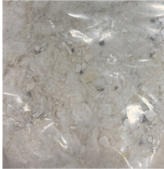
Figure 10: Shredded boat fibers consisting of 33% glass fiber and 66% epoxy.
