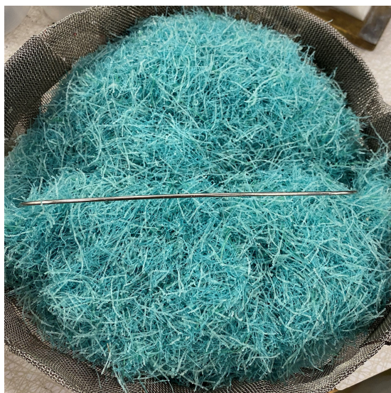
Figure 3: Shredded and dried fishing nets before compounding
