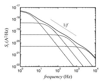
Figure 2.4. Superposition of four Lorentzians which exhibits a 1/f dependence. Figure taken from [12].
