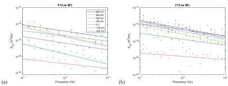
Figure 5.4 (a) (b) PSD vs frequency for two devices on the 2834-sample(w SF)
