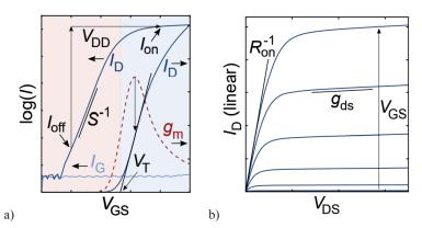
Figure 2.2 (a) Transfer characteristics. Drain current vs gate voltage. (b) Output characteristics. Drain current vs drain voltage. Figure taken from [1].
