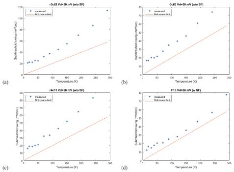
Figure 5.3 (a) (b) (c) SS (mV/dec) vs temperature at  $V_{DS}$ =50 mV for device r3c62, r3c63 and r4c11 respectively, on the 3738-sample(w/o SF). Devices r3c63 and r4c11 broke during and before the last measurement at 290 K which is why those data points are below the theoretical limit. (d) SS (mV/dec) vs temperature at  $V_{DS}$ =50 mV for device F13 on the 2834-sample(w SF).
