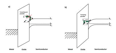
Figure 2.5. Band diagrams of biasing of trap states. (a) Lower  $V_{GS}$ , trap states not close enough to the Fermi level for tunnel transitions to occur. (b) Higher  $V_{GS}$ , trap states are closer to the Fermi level and tunneling transitions are more likely to occur.
