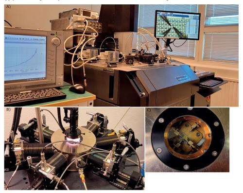
Figure 4.1 (a) The Semi-auto probe station (the black box with all the cables) and the parameter analyzer (on the left) (b) The cryo probe station (c) The inside of the cryo chamber with three probes connected to one device.
