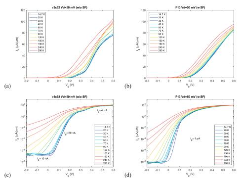
Figure 5.1 (a) (b) transfer characteristics at different temperatures for device r3c62 on sample 3738(w/o SF) and device F13 on sample 2834(w SF) respectively, at  $V_{DS}$ =50 mV and in linear scale. (c)(d) transfer curves at different temperatures for the same devices and at  $V_{DS}$ =50 mV but in logarithmic scale. It can be seen that the current decreases with decreasing temperature and that the threshold voltage increases with decreasing temperature for both devices.
