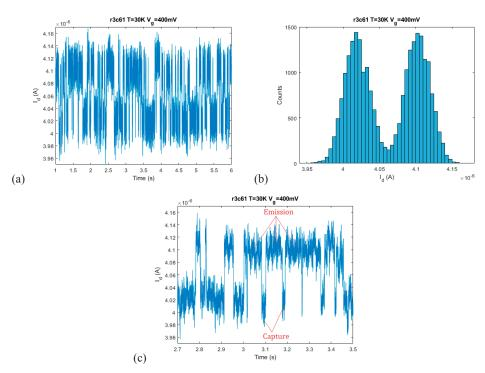
Figure 5.9. (a) RTS noise of sample 3738(w/o SF) (b) Current histogram of (a) (c) Zoom in on (a) showing the capture and emission parts.
