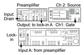
Figure 4.2. Schematic of LFN measurement setup, taken from [1].
