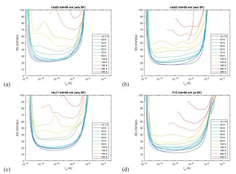
Figure 5.2 (a) (b) (c) SS (mV/dec) at different temperatures with  $V_{DS}$ =50 mV for device r3c62, r3c63 and r4c11 respectively, on the 3738-sample(w/o SF). (d) SS (mV/dec) at different temperatures with  $V_{DS}$ =50 mV for device F13 on the 2834-sample(w SF).
