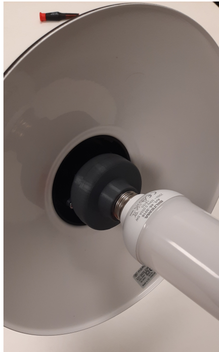
Figur 8.9 The casing is mounted to the lamp house
