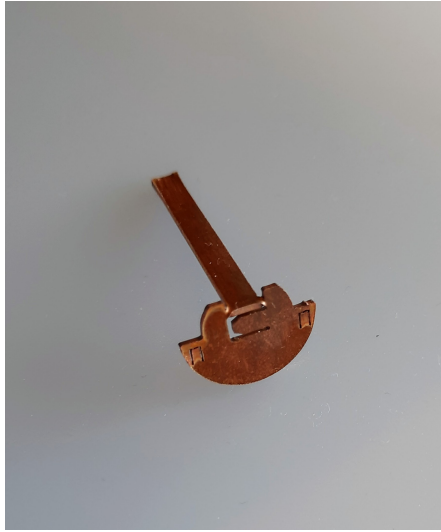
Figur 5.4 An early design of the 1mm active contact metal which has been laser cut and then bent by hand.
