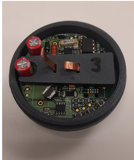
Figure 8.4 The opened casing with the bridge in place
