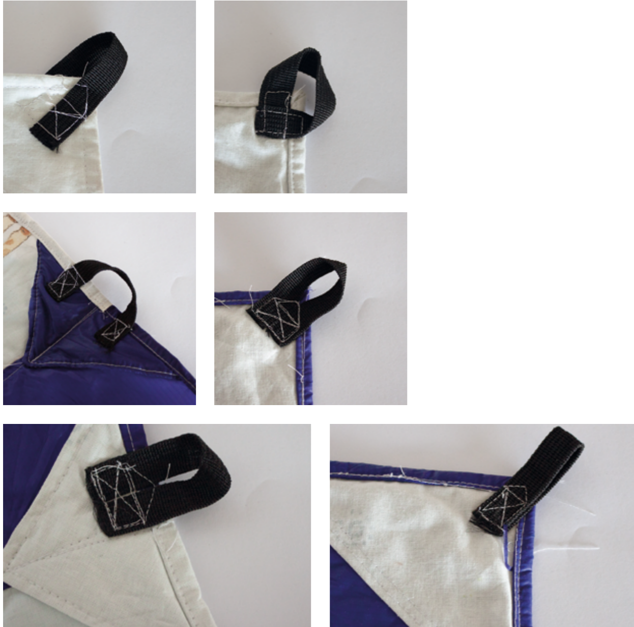
Trying out different options for eyelets to fasten the tarp. Finally, I decided for the both eyelets in the bigger pictures. On the left side it is the eyelet for the sides. On the right side is the eyelet for the edges as this worked the best in combination with the buckles.
