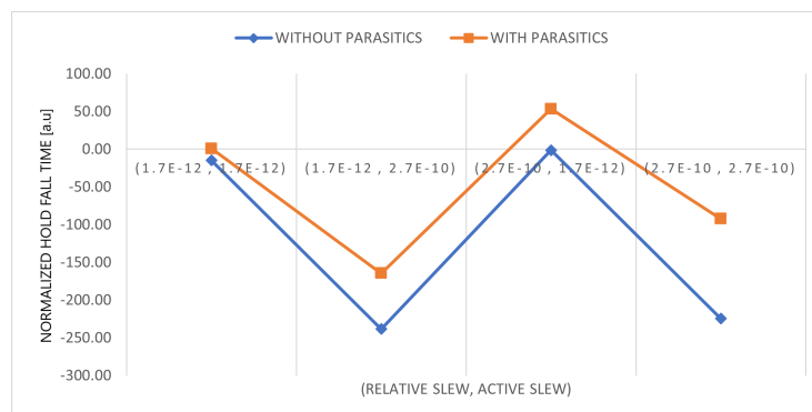
Figure 7.4: Hold Fall time variation with layout parasitics
