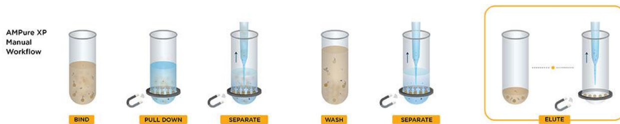
Figure 3 Workflow of AMPure XP Bead Cleanup in final microbiome DNA enrichment step (Beckman Coulter Life Sciences, AMPure XP Workflow . 2022).
