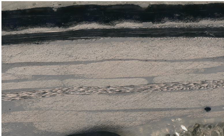
Fig. 33: Magnified version of figure 32 showing the stacking sequence more clearly. To distinguish the different plies one should use the same principles as presented in figure 30.
