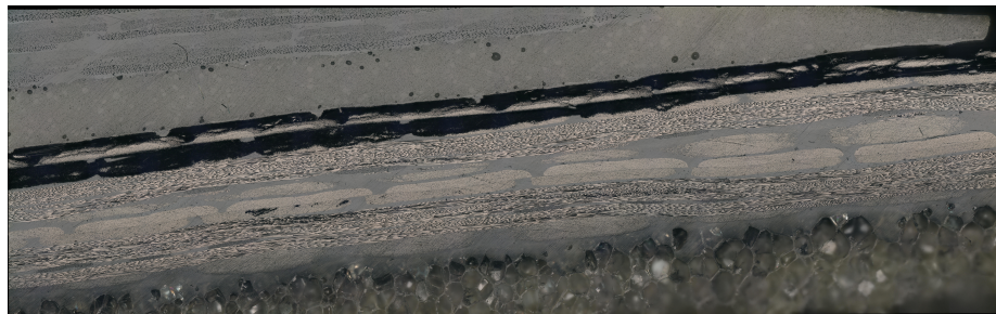
Fig. 29: Image of the S45 sample after the second and final polishing sequence. The topmost fibers of this sample is at a 45 degree angle with the examined surface, the second ply is also at a 45 degree angle with the examined surface and the three following plies are parallel with the examined surface.
