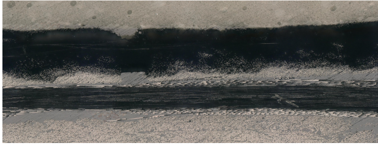
Fig. 34: S90 sample magnified even further than figure 33 to show how the bundles of the topmost carbon fiber ply has stayed together unlike the bundles from figure 31. Even the resin-rich connections between individual bundles are relatively intact.
