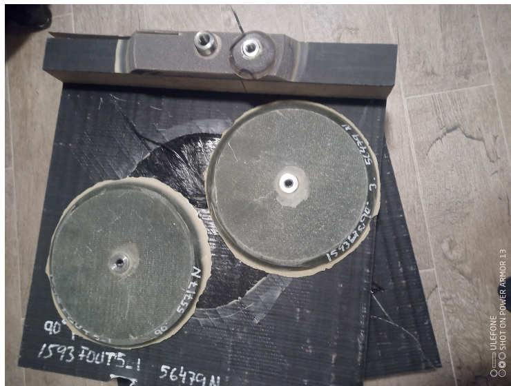
Fig. 17: Two specimens can be seen in this image, they are the two sandwich panels stacked on top of each other along with their two large glass fiber patches. These pieces were separated during tensile testing of the patches. The specimen that was used for the microscopic analysis in this report is the bottom sandwich panel and the patch with the number 55717 (the fracture load). At the top of the image is the test sample, from figure 1a and 1b, that was used in the microscopic evaluation.
