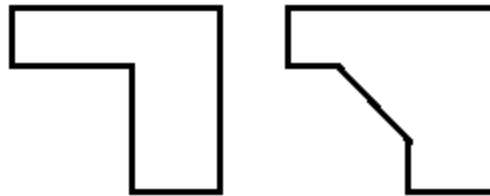
Figure 35: Difference between a support angle of 90° and 45°
