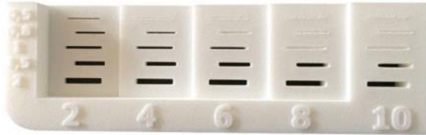
Figure 18: Hole size depends on material thickness [26]
