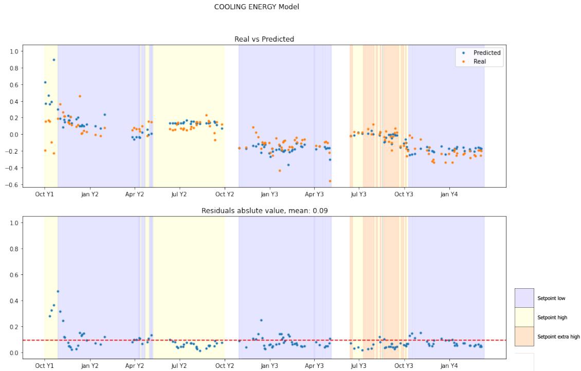
Figure 4.11: Cooling model, predictions on the test-data
