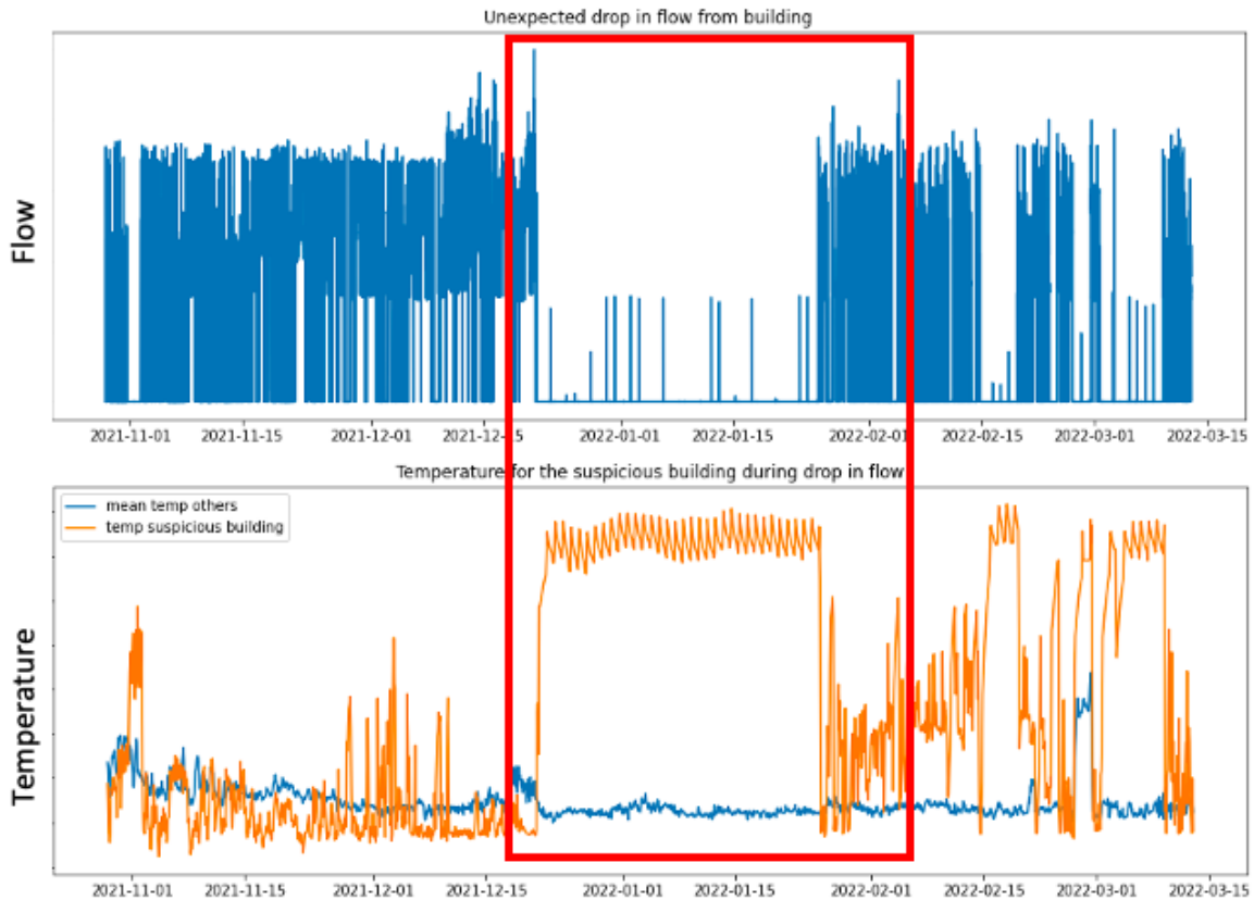
Figure 3.2: An unexpected drop in flow from one of the buildings (top) with a simultaneous raise in temperature in the same building (bottom).
