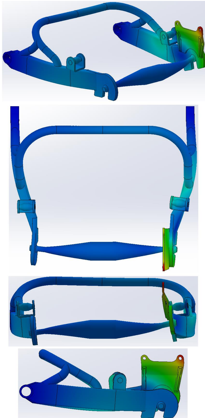
Figure C.6 The displacement results from the hard braking case, high crossbar variant. Deformation scale 154. The reddest node moved 0,321 mm.
