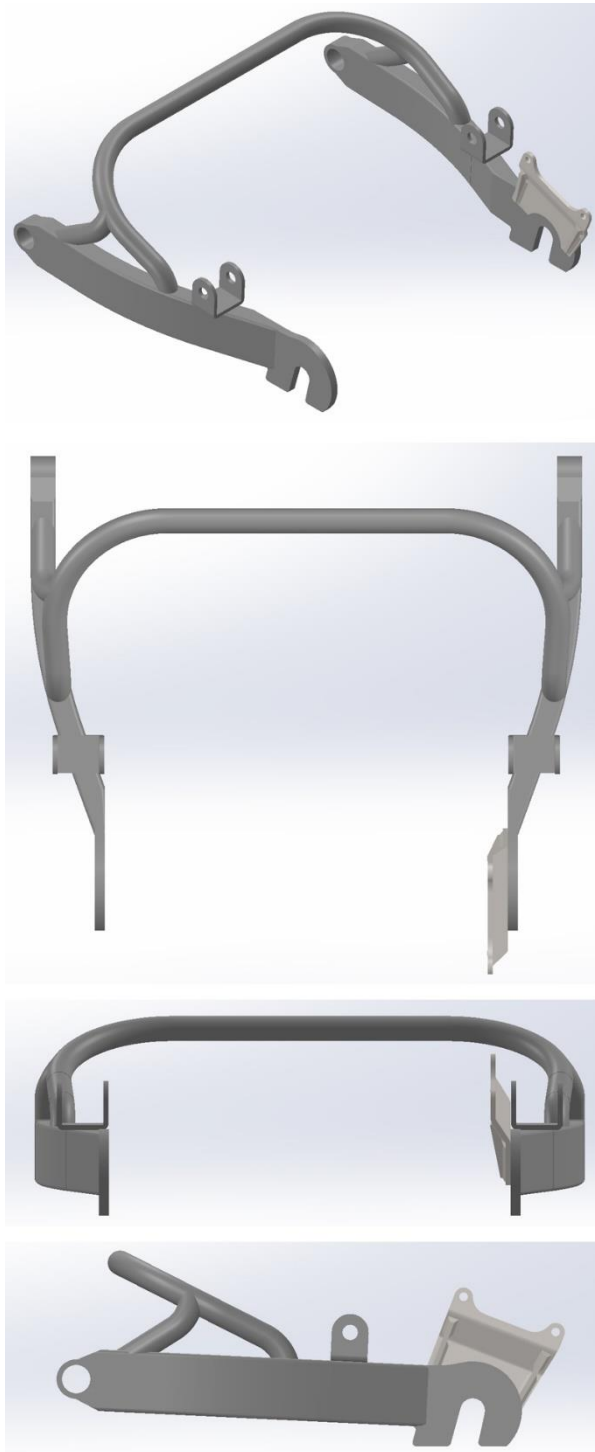
Figure 7.7 The final design of the high crossbar variant. Views: angled, top, back, left.
