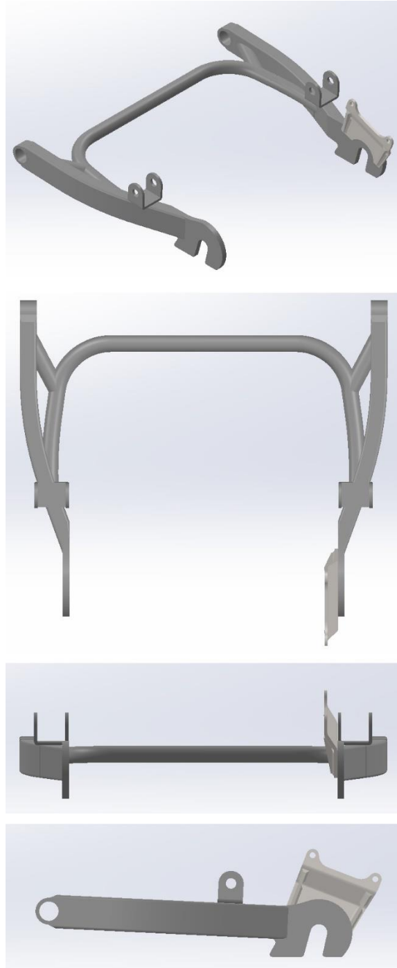
Figure 6.4 The initial design of the flat crossbar variant. Views: angled, top, back, left.
