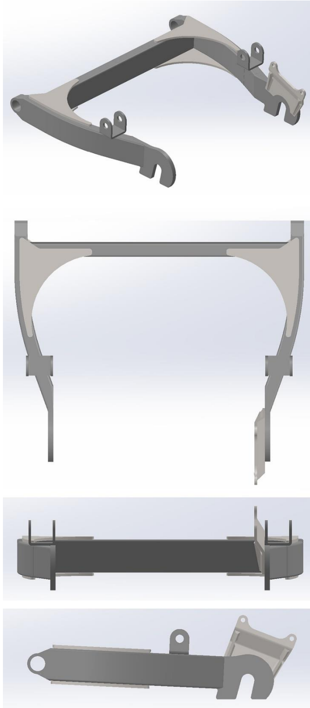
Figure 7.8 The final design of the flat crossbar variant. Views: angled, top, back, left.
