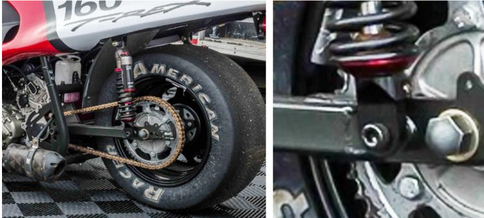
Figure 10.2 The bolt fastening configuration on the lateral face of the swingarm used on some Campagna T-Rex models (adapted from [27]).
