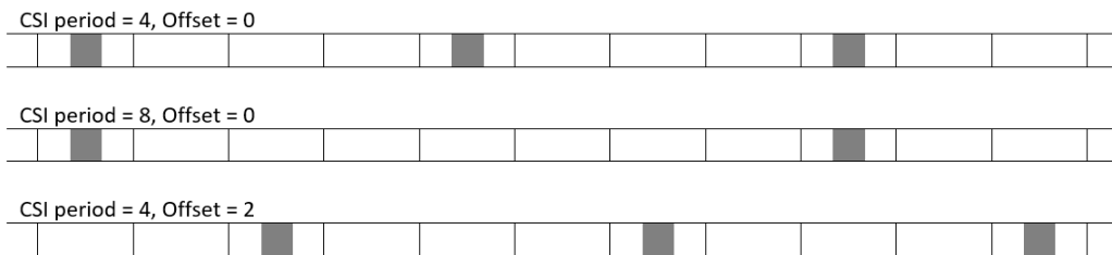
Figure 4.6: Examples of periodic CSI-RS and slot offset
