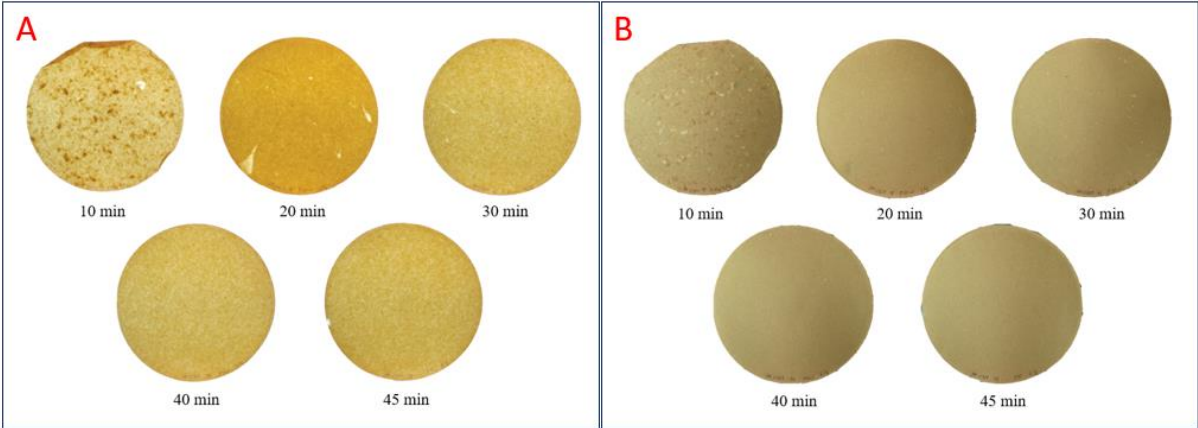
Figure 10. Sheets made from PM A run with standard parameters, taken at 10, 20, 30, 40 and 45 minutes of pulping. Photographed with light from behind (A) and from the front (B).
