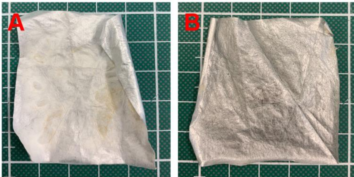
Figure 9. PM with (A) and without (B) the laminate intact on the PolyAl.
