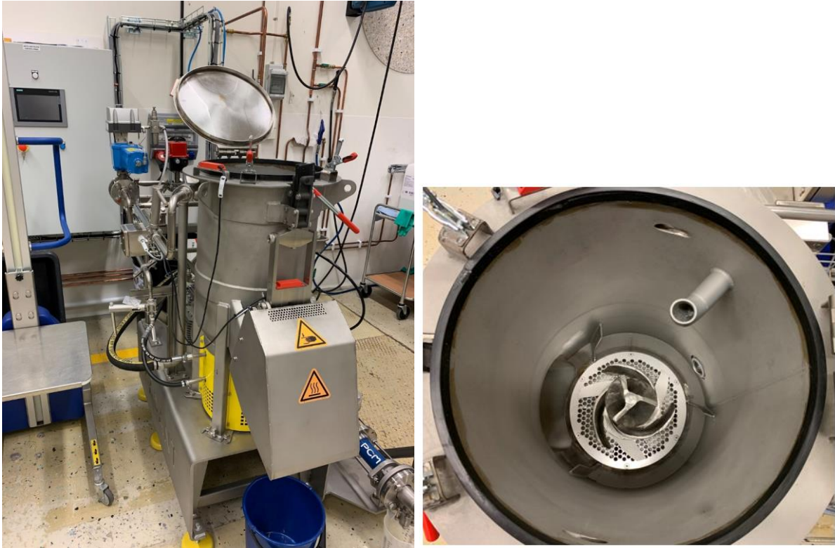
Figure 7. The high consistency (HC) Pulper.
