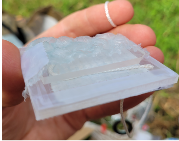
(b) Finalized chip with support structures ready to be installed in the field. The exposed chip entrance is facing the camera. Support PMMA bottom, bubble wrap, and string with metal ring can be seen.
