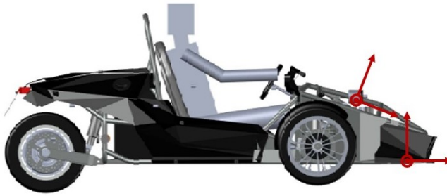
Figure 5.1 Displacement between gyroscope and accelerometer coordinate system
