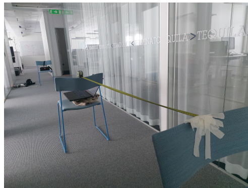
Figure 3.7: First manual data gathering method using chairs and measuring tape.
