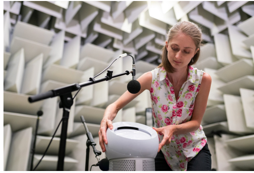
Figure 2.1: A example of a anechoic chamber [24].
