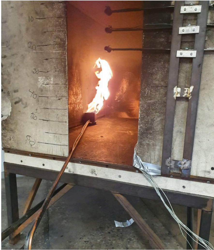
Figure 34: Flames not sticking to the wall at 10 kW after 10 minutes, potentially due to airflow.
