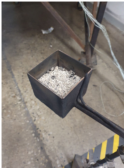
Figure 12: Gas burner filled with sand.
