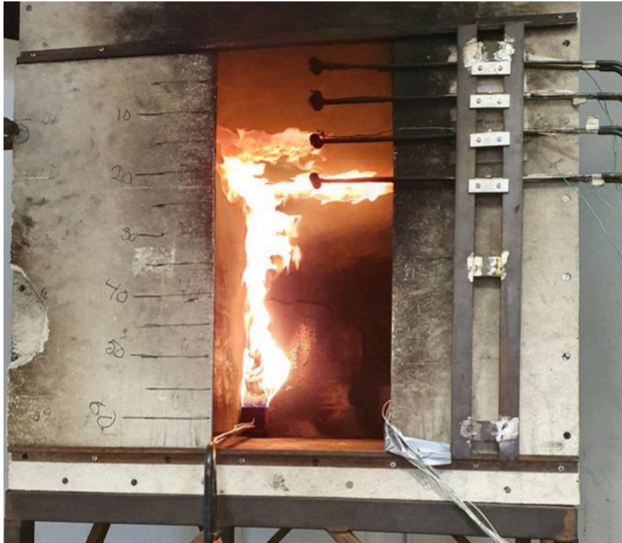
Figure 33: Flame height from gas experiment 1 sticking to corner and extending below the ceiling at 20 kW after 10 minutes.
