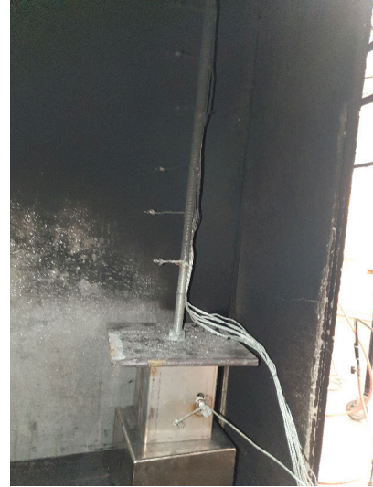
Figure 15: Thermocouple tree in the right corner of the room.
