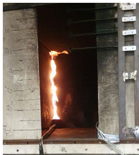
Figure 32: Flame height from fire in the corner with gaseous propane at 5 kW.
