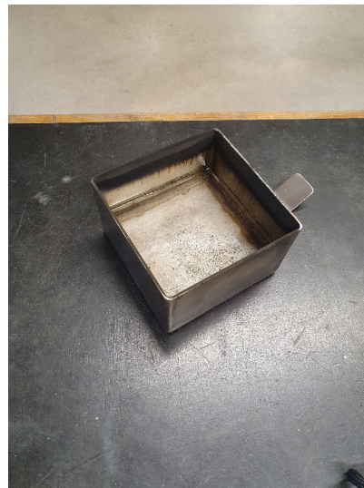
Figure 13: Container for liquid fuel with water to get a higher flame base.
