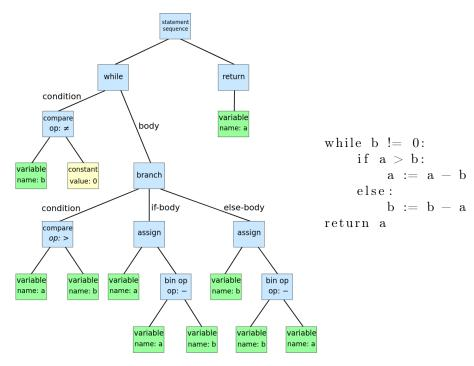
**Figure 5.1:** Abstract syntax tree for the Euclidean algorithm to find the greatest common divisor of a and b alongside the corresponding pseudocode [20]
