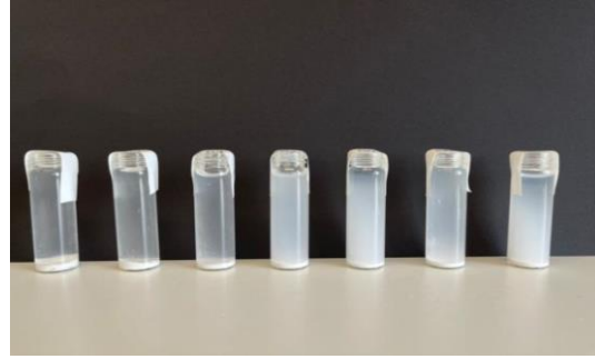
Figure 15. Suspension photos of the HA3 pellets in water: (A) HA3 with SC; (B) HA3 with WPI. From left to right, the protein concentration increased. The first one on the left is the control group without adding protein.
