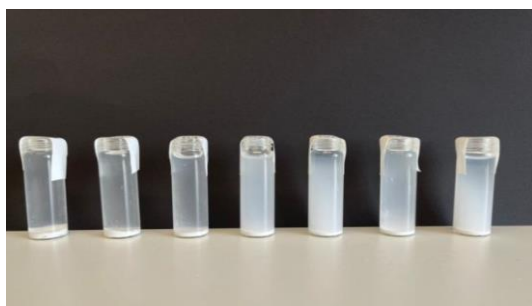
Figure 17. Suspension photos of the Capolac pellets in water: (A) CA with SC; (B) CA with WPI. From left to right, the protein concentration increased. The first one on the left is the control group without adding protein.
