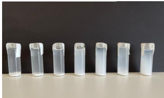
Figure 7. Suspension photos of the three batches of HA powders: (A) HA1 suspended in SC; (B) HA1 suspended in WPI; (C) HA2 suspended in SC; (D) HA2 suspended in WPI; (E) HA3 suspended in SC; (F) HA3 suspended in WPI. From left to right, the protein concentration increases. The first sample on the left is always the control group with water.
