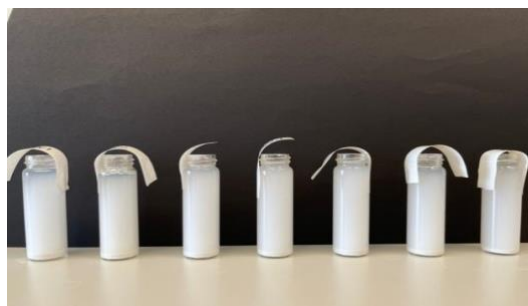
Figure 17. Suspension photos of the Capolac pellets in water: (A) CA with SC; (B) CA with WPI. From left to right, the protein concentration increased. The first one on the left is the control group without adding protein.
