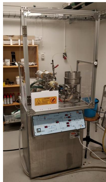
Figure 7: Schematic of the basic principle of a pasteurizer along with an image of the Armfield pasteurizer used in this thesis.
