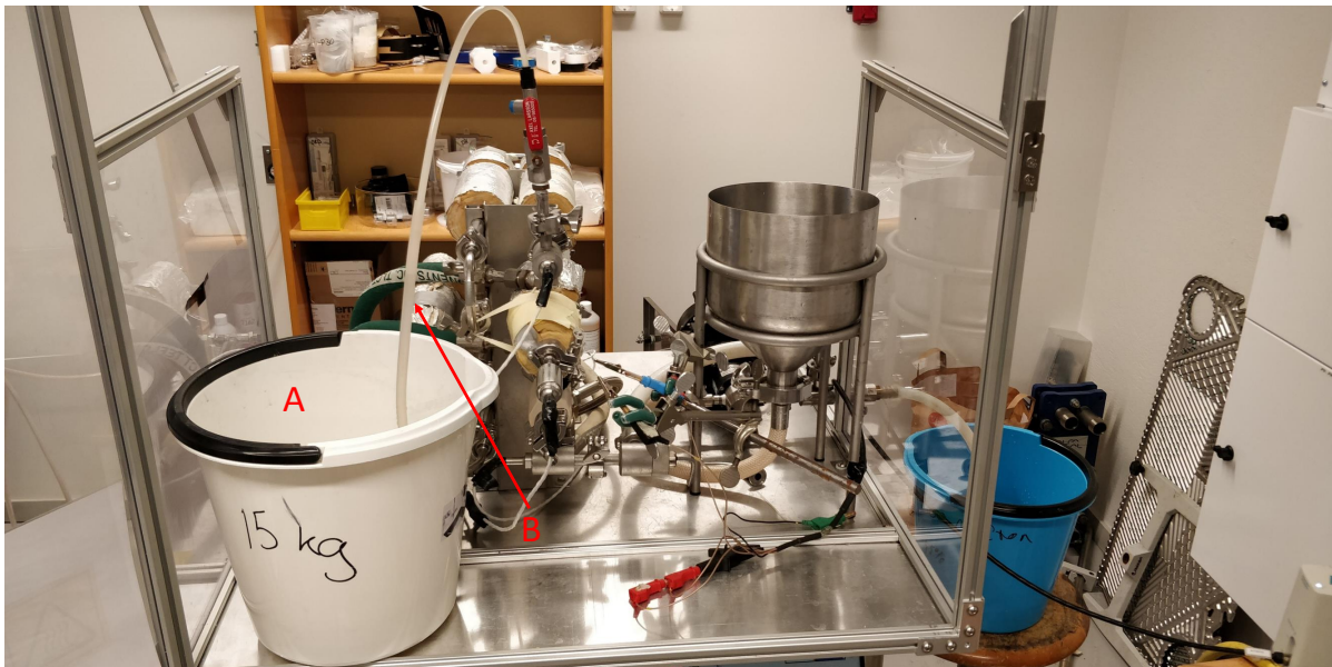
Figure 29: Image of the cleaning setup for Sören. The "re-feeding" tube, showcased by B should be put into a bucket so as to not reuse old water. A just points towards an ordinary bucket used as a container for the dirty water.
