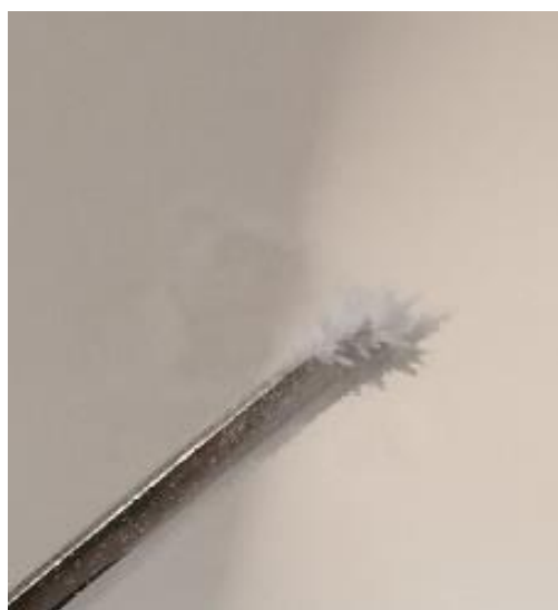
Figure 23. Formulation observed exhibiting electrostatic effects when handled with a spatula.
