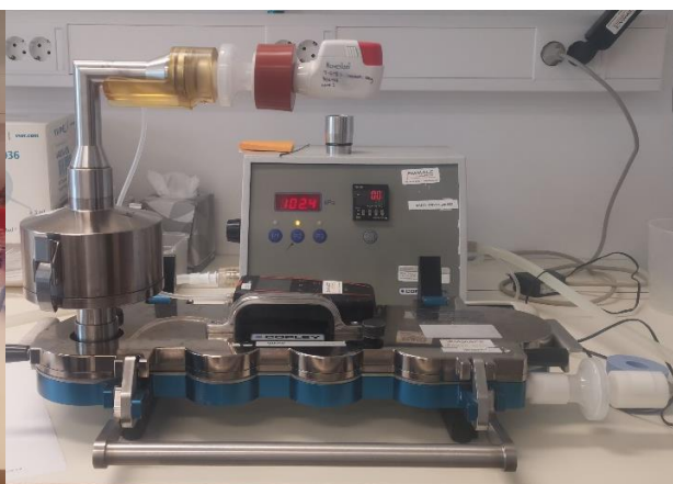
Figure 16. Picture of the NGI setup used.
