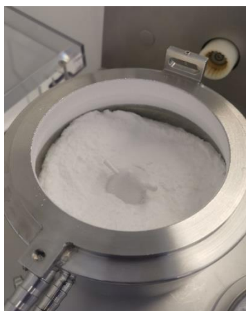
Figure 10: Picture of the Diosna mixing vessel containing formula.
