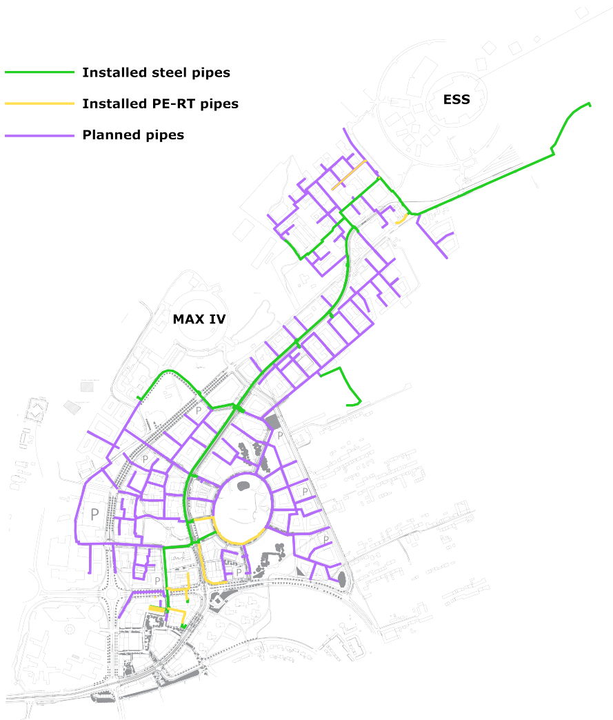
Figure 3.2 A map of the district heating network in Brunnsbög, with the installed steel pipes in green, the installed PE-RT pipes in yellow, and the planned pipes in purple. The steel pipes provide the main path from the supply at MAX IV, while the plastic pipes service the individual buildings.
