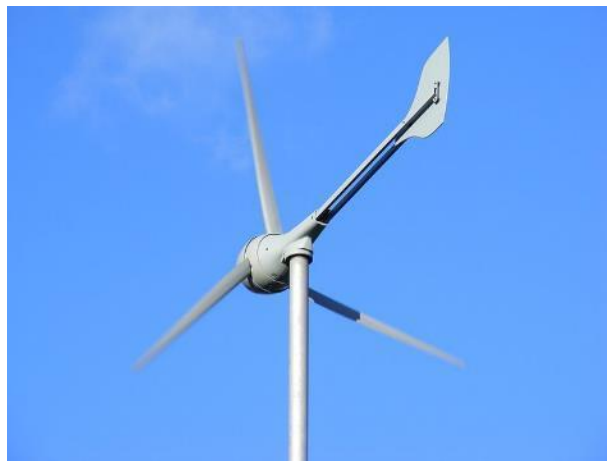
Figure 3. Photograph - Evance HAWT R9000 5kW small wind turbine. Photo – Tobi Kellner March 2013 (Creative Commons Attribution-Share Alike 3.0 Unported license https://creativecommons.org/licenses/by-sa/3.0/legalcode )
