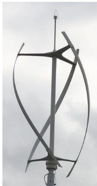
Figure 4. Photograph - Gorlov Turbine - Helgoland, micro wind turbine "QR 5" Photo- Sozialutopist August 2012 ((Creative Commons Attribution-Share Alike 3.0 Unported license https://creativecommons.org/licenses/by-sa/3.0/legalcode )
