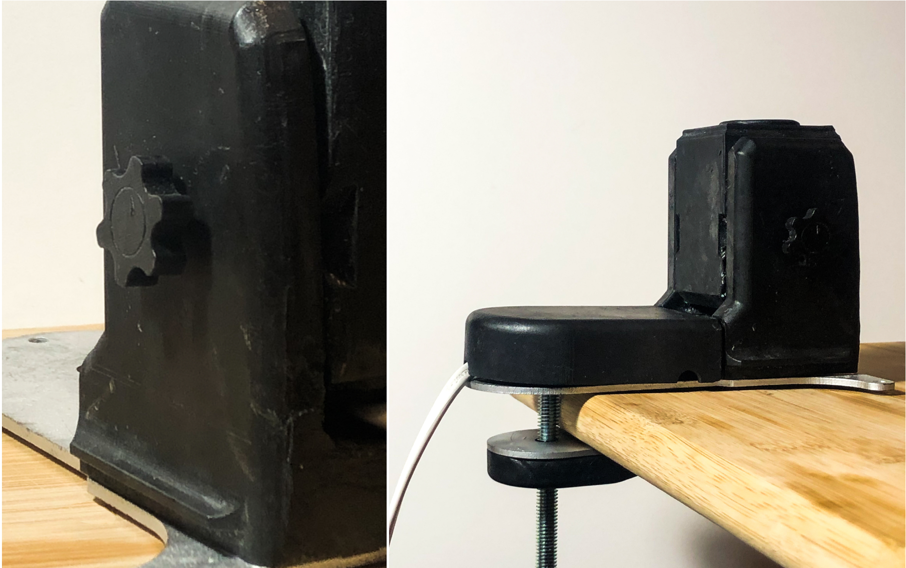
Detailed photos highlight the poor quality of the resin print. This prototype was not sufficient as a final result.
