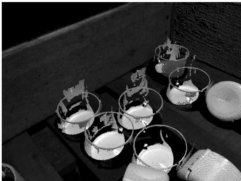
Figure 5.5 Example of errors in point cloud reconstruction due to interreflections
