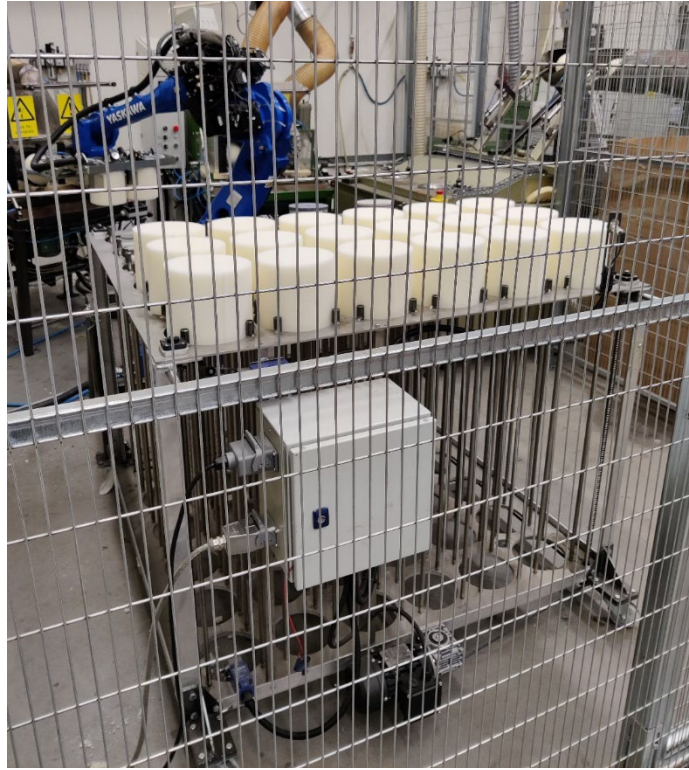
Figure 7.6 The Cylinder magazine inside the enclosure. The magazine can be pushed with the help of wheels underneath.
