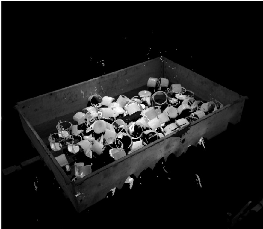
Figure 5.4 Scan of a bin filled with cups. Above the bin, floating point artifacts can be seen.
