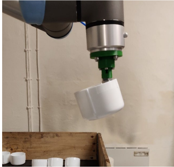
Figure 5.10 Tilt as a result of the convex surface on the inside of the cup.
