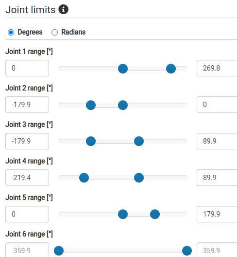
Figure 4.12 Image depicting the final joint limit settings. Joint 1 refers to the joint of the base while joint 6 controls the rotation of the toolflange joint.
