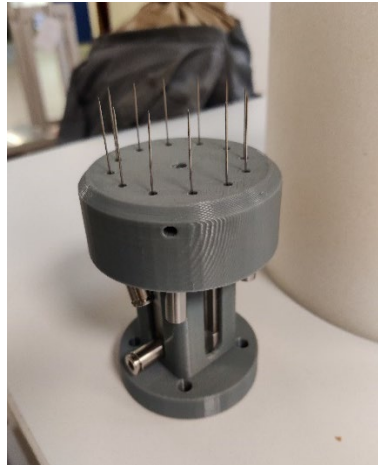
Figure 3.12 Image depicting the complete needle gripper while the cover is retracted.
