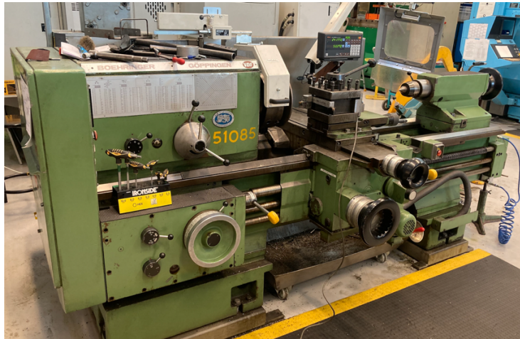
Figure 31. Boeringer Göppingen VDF lathe used in the machining tests.
