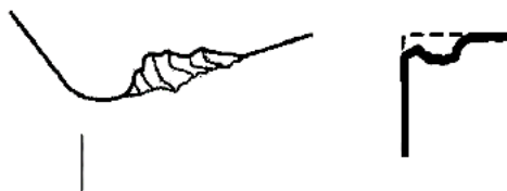
Figure 13. Depiction of mechanical fatigue cracking [10].
