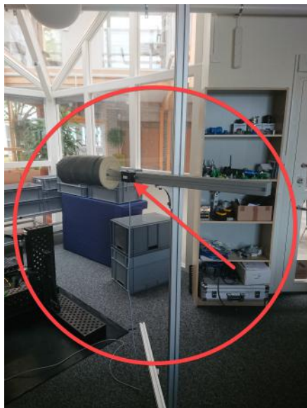
Figure 4.1 Close look at the construction of the collision obstacle. The red circle encircles the whole collision object and the red arrow points at the accelerometer used to get a reference signal.
