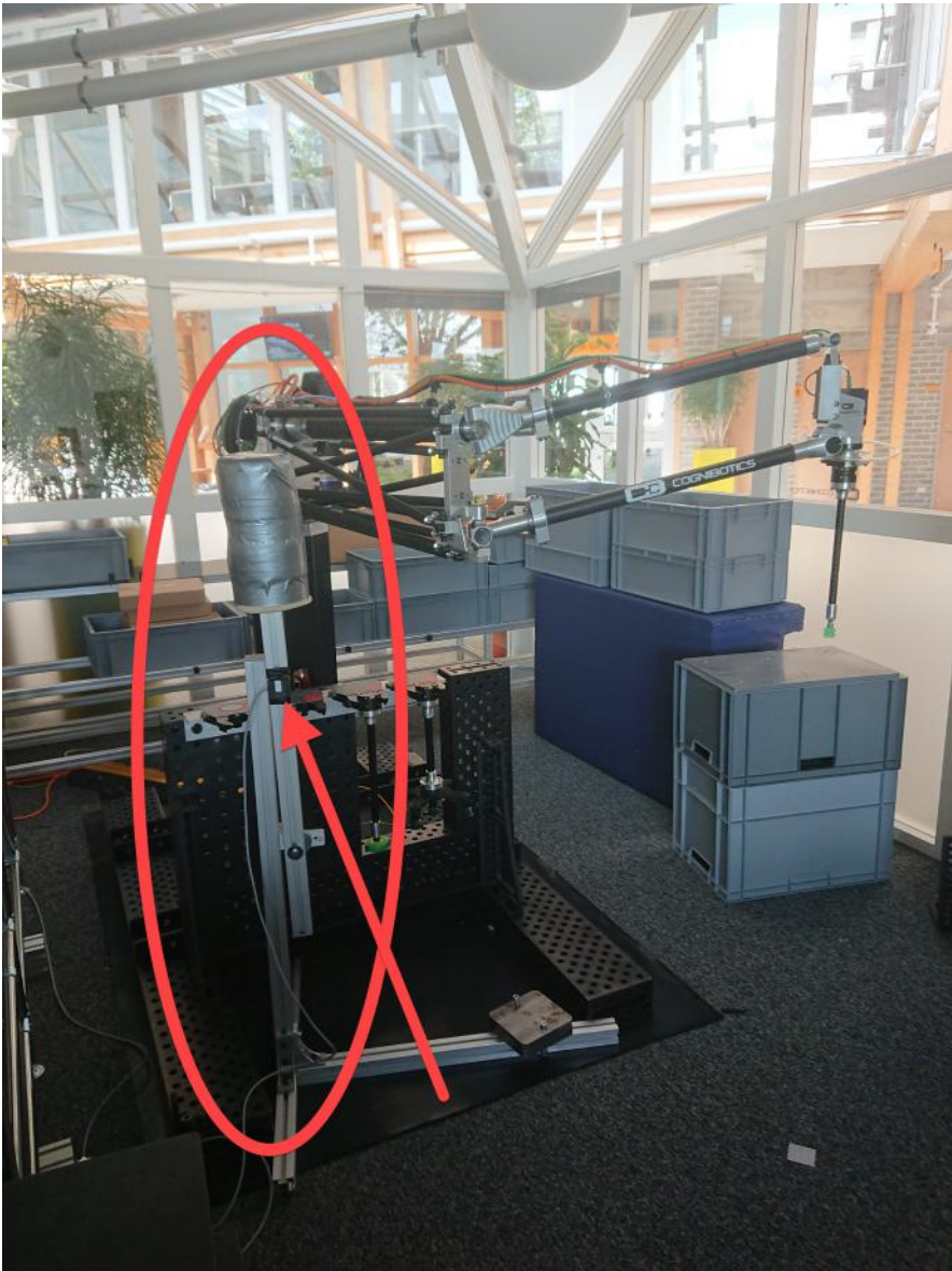
Figure 4.3 Overview picture of the reconstructed collision obstacle for inner collisions and the robot. The red circle encircles the reconstructed collision object and the red arrow points at the accelerometer that gives the reference signal.
