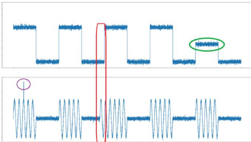
Figure 3.1 Illustration of different types of anomalies. A point anomaly (purple), contextual anomaly (red) and collective anomaly (green) [Audibert et al., 2022].
