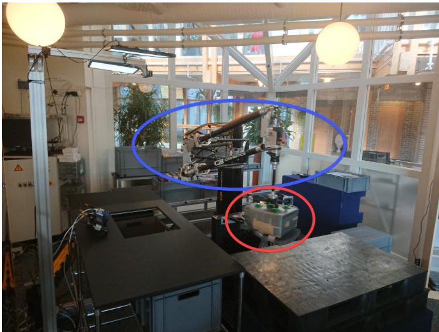
Figure 4.5 Overview picture of the robot carrying the object used in object drop experiments. The blue circle encircles the HKM robot, and the red circle encircles the object used for the experiment.
