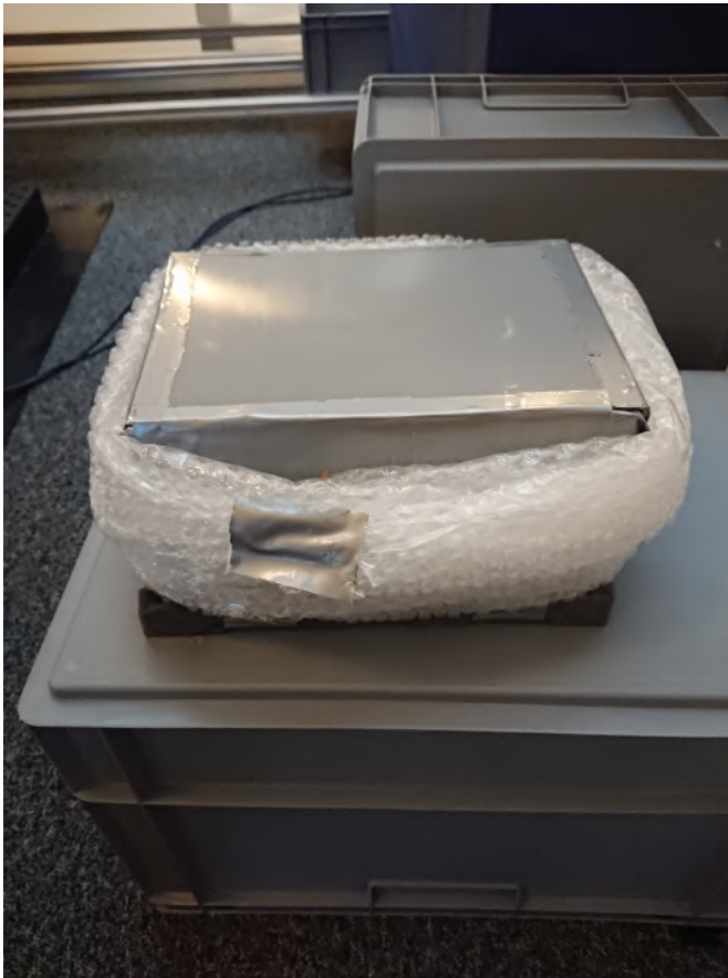
Figure 4.4 Close look at the object used for drop experiment, in this picture the lid used for the heavier load of 7.5 kg is on.
