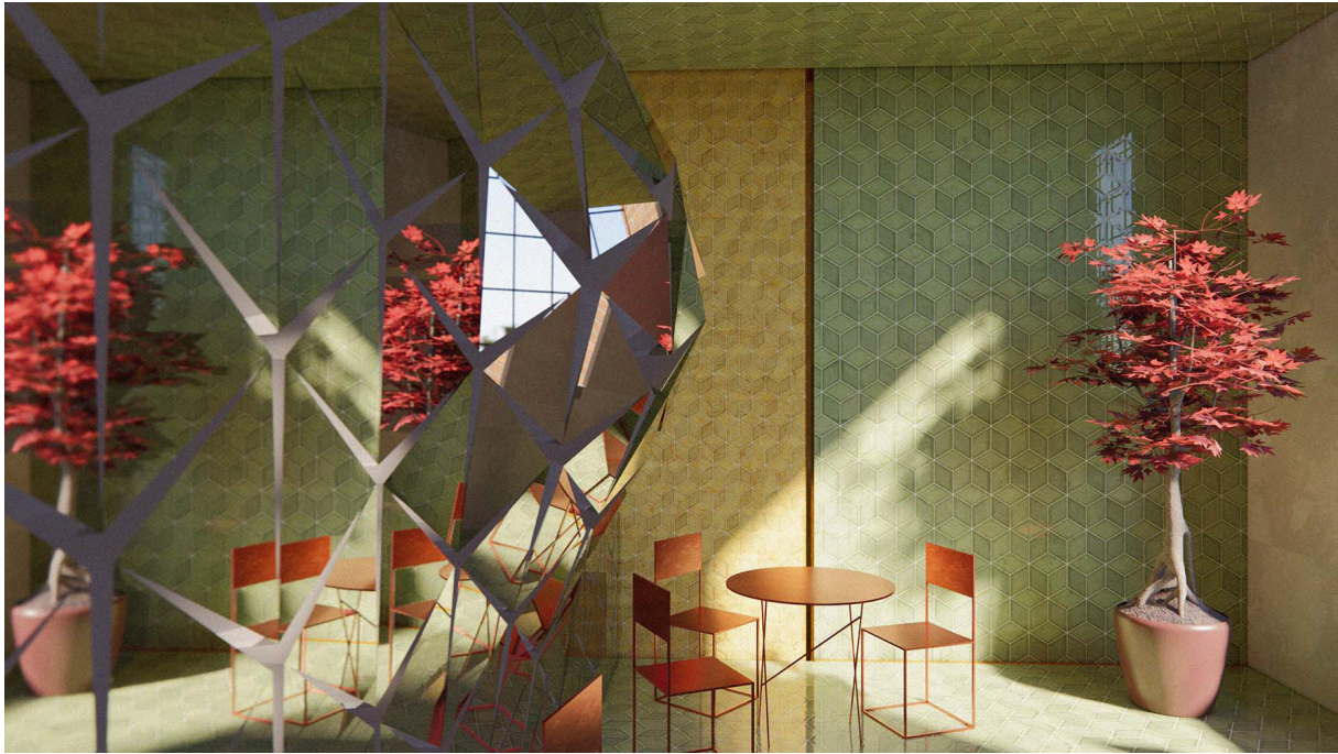
Visualisation of wall elements where reflective mirrors are attached to the origami surface
