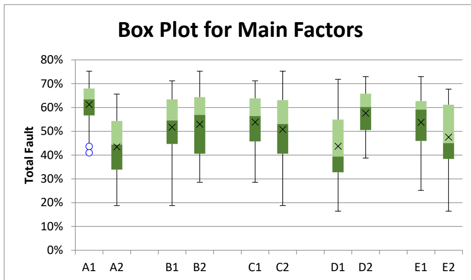
Figure 5.4 To further investigate the significance of main factor a box plot was made. The individual plots show the mean value as an x. The upper and lower quartiles in green. Maximum and minimum bounds indicate maximum and minimum values for each group, except outliers marked with a blue circle.
