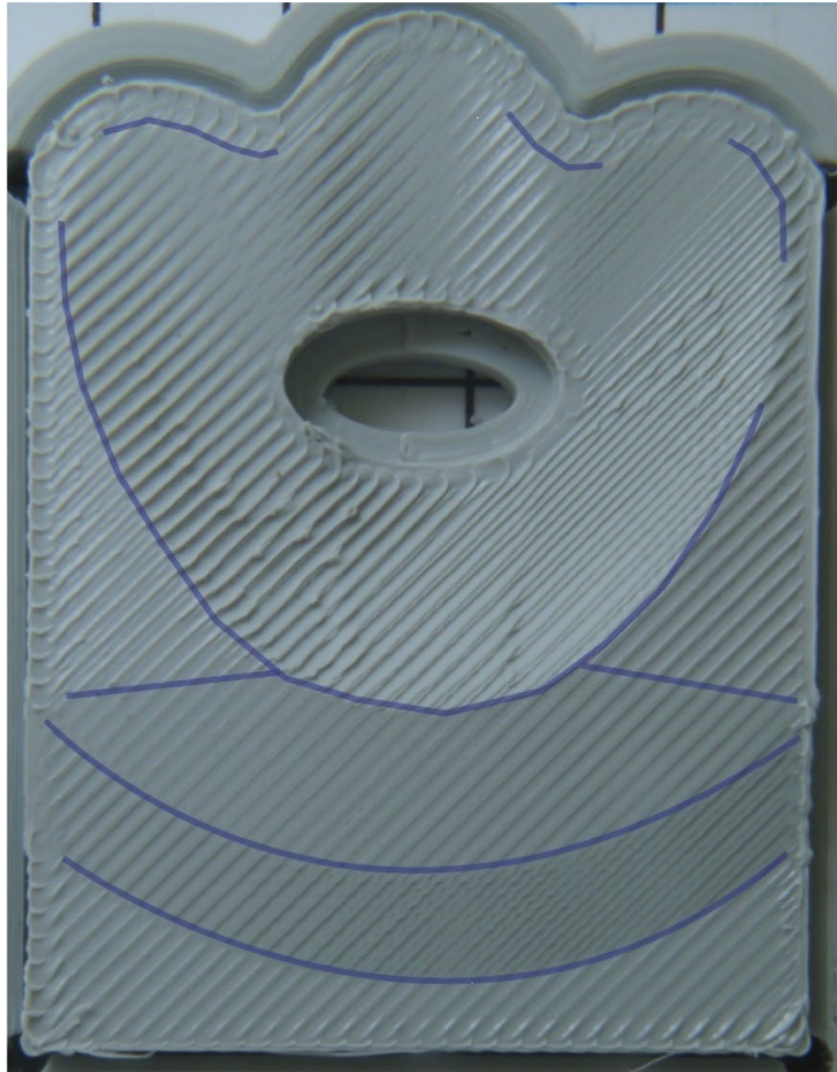
Figure 4.2 The picture shows what areas of the part has defined lines between the different surfaces of the model, marked in blue. This was compared to the 3d-models values for the perimeter length projected to a 2d.
