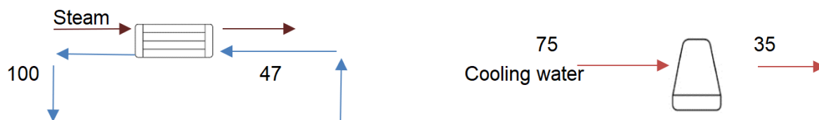
Figure 13: Sketch of a district heating design where heat in the cooling water is not utilized.
