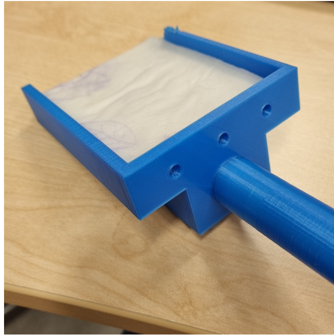
Figure 36: (Passively) water cooled phone holder, which significantly helped cool the phone during measurements
