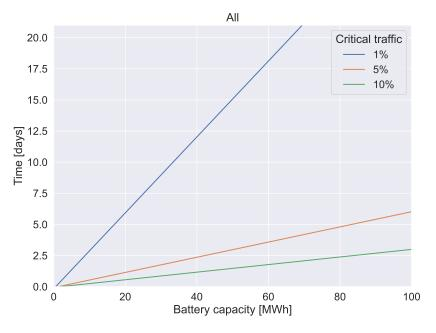
**Figure 4.13:** Number of days during which some fractions of the flow of All traffic can be sustained with a given ESS capacity.
