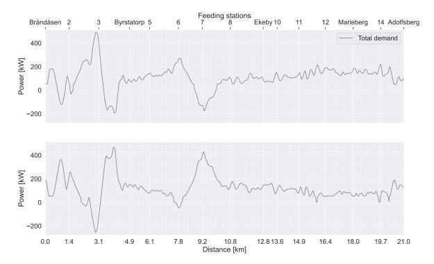
Figure 3.5: The truck with trailer's power demand over the distance, one plot for each direction
