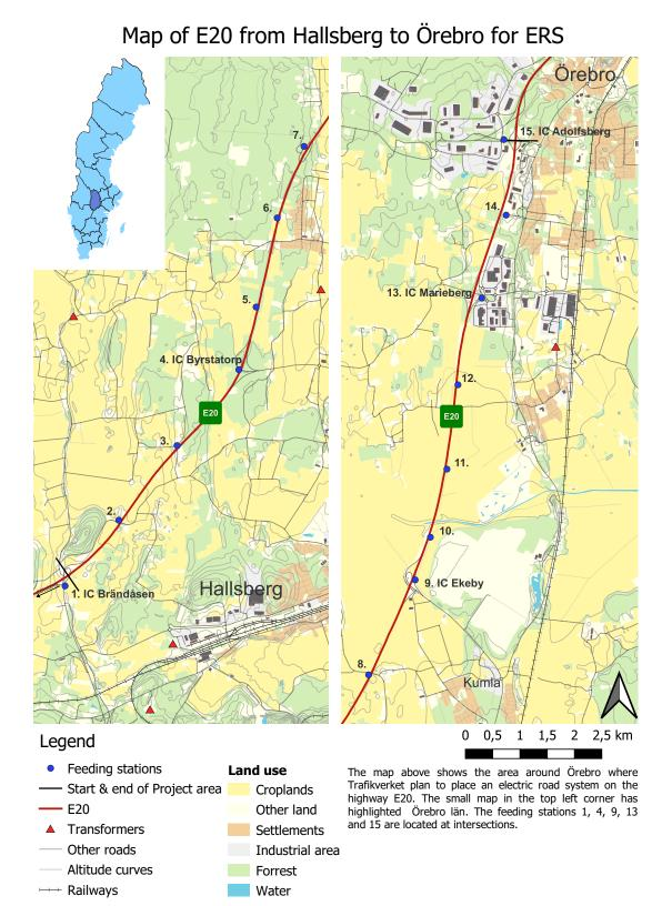
**Figure 2.1:** Map of the Project area with the ERS and its feeding stations marked. Created using QGIS with maps from Swedish University of Agricultural Sciences (2022).
