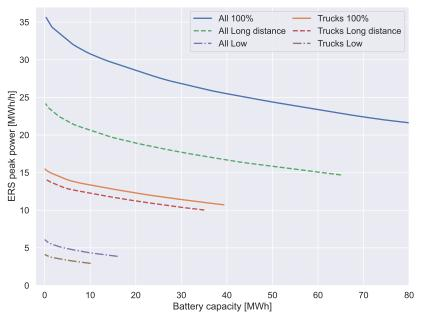
Figure 4.15: ERS peak power vs. battery capacity for All traffic and Trucks for three different scenarios
