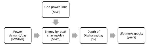
Figure 3.7: Flowchart of the lifetime model for peak shaving
