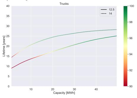
**Figure 4.8:** ESS lifetime vs. battery capacity for Trucks for two power limits. The color bar shows percentage of days during which the capacity is sufficient for peaks shaving.
