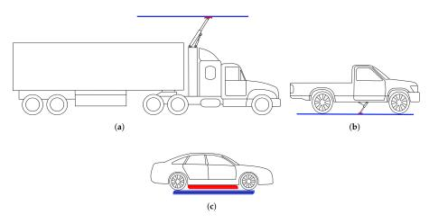
**Figure 2.3:** Three types of ERS technologies. Modified from Domingues-Olavarría et al. (2018) with permission.
