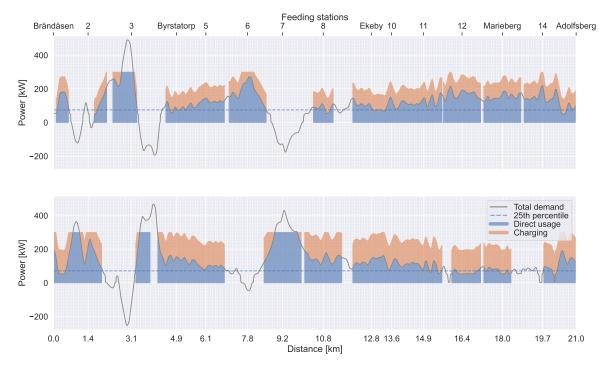
**Figure 4.3:** The truck with trailer's power demand over the distance, one plot for each direction
