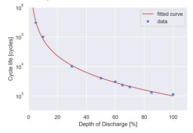
**Figure 3.8:** Cycle life as a function of depth of discharge shown as a fitted curve and real data, the data is taken from (GWL, 2015)
