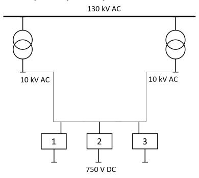
Figure 3.6: Model of the power system
