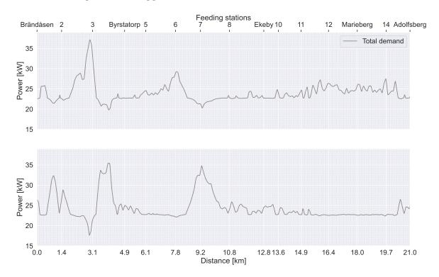
Figure 3.3: The car's power demand over the distance, one plot for each direction
