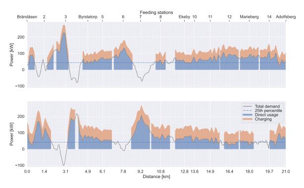
Figure 4.2: The truck without trailer's power demand over the distance, one plot for each direction
