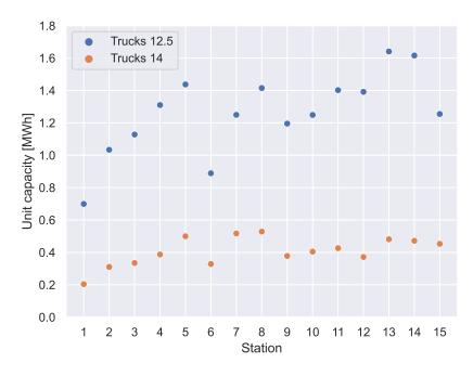
**Figure 4.10:** ESS capacity need for the different feeding stations when Trucks use the ERS.
