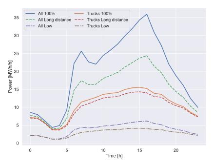
Figure 4.14: Power demand (95th percentile) over the day for All traffic and Trucks for three different scenarios
