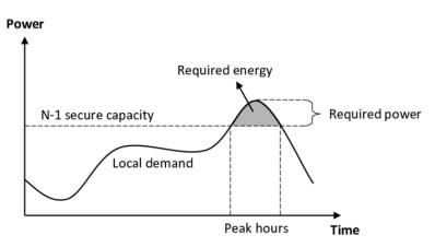
Figure 2.5: Example of peak shaving with ESS over a day (Strbac, Konstantelos, and Djapic, 2016)
