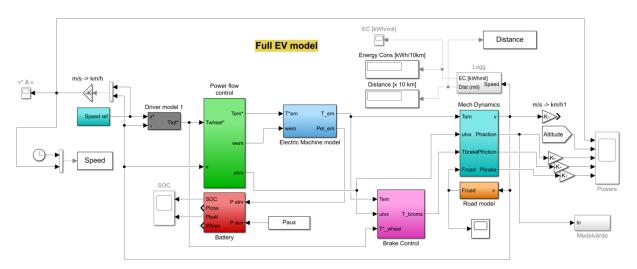
Figure 3.2: Overview of the electric vehicle Simulink model
