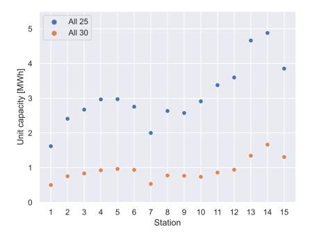
**Figure 4.11:** ESS capacity need for the different feeding stations when All traffic uses the ERS.
