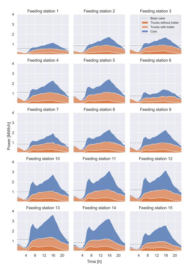
Figure 4.4: Power demand (95th percentile) for each feeding station
