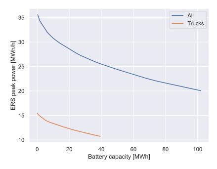
Figure 4.6: Change in ERS peak power as a function of ESS capacity used for peak shaving
