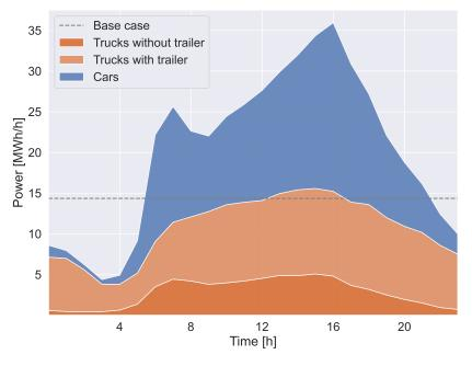
Figure 4.5: Power demand for all the feeding stations aggregated
