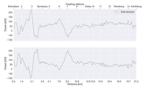
Figure 3.4: The trucks without trailer's power demand over the distance, one plot for each direction
