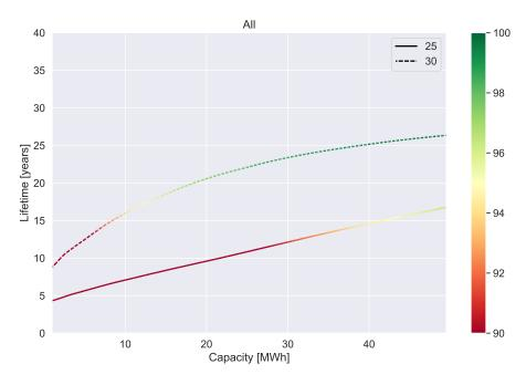
**Figure 4.7:** ESS lifetime vs. battery capacity for All traffic for two power limits. The color bar shows percentage of days during which the capacity is sufficient for peaks shaving.
