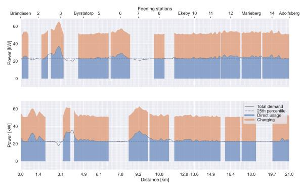
Figure 4.1: The car's power demand over the distance, one plot for each direction
