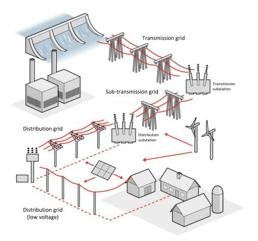
**Figure 2.4:** The Swedish power transmission system. Modified with permission from Energiföretagen (2021)
