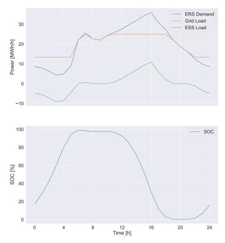
**Figure 4.9:** Peak shaving example using All traffic, a power limit of 25MWh/h and a ESS capacity of 45MWh. Upper graph shows power demand, lower shows corresponding SoC.
