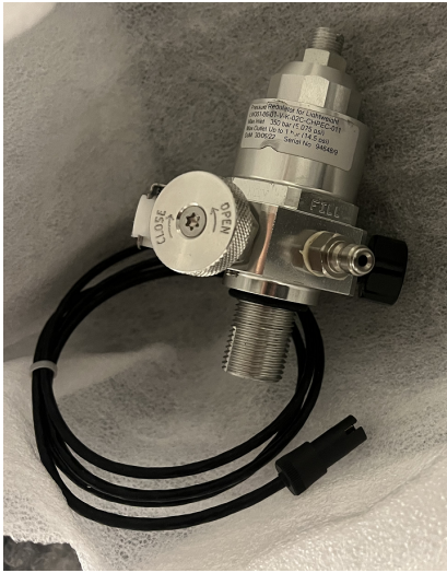
Figure 7.5.: The H3Dynamics-provided hydrogen pressure regulator. Visible is the main valve and the connector for filling. The regulator is threaded in order to be screwed into the hydrogen cylinder.
