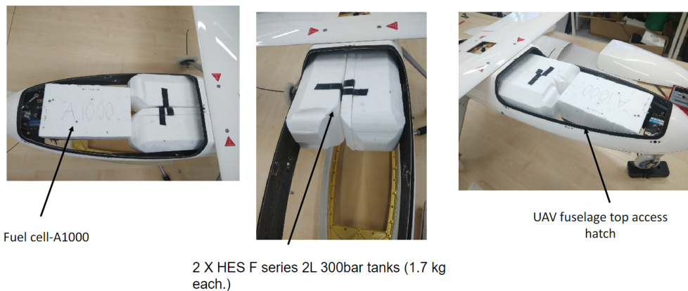
Figure 3.5.: Images of the styrofoam cutouts made to test how the fuel cell system may be integrated in the airframe.
