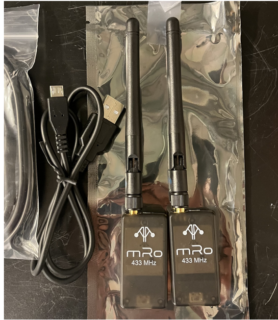
Figure 6.2.: The two wireless transceivers used to transmit telemetry data from the AeroStak to the controller PC.
