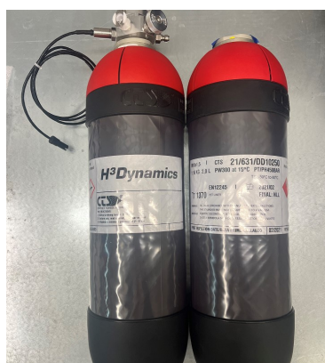
Figure 3.6.: The two high pressure cylinders to be used for storing hydrogen onboard the UAV.
