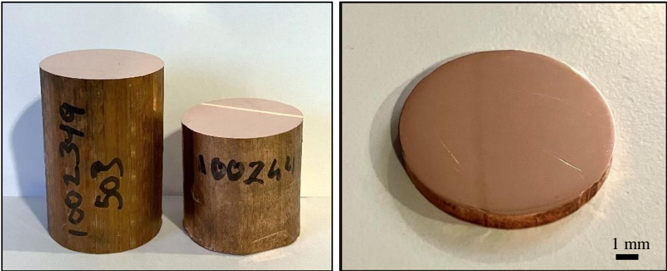
Figure 4.2. Examples of 30 mm CuMg0.49 coil samples before sample preparation. Some scratches from the grinding procedure are observable.
