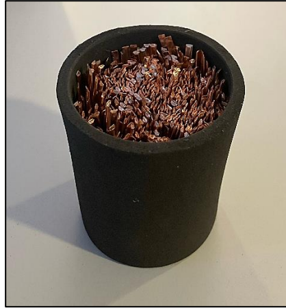
Figure 4.3. Graphite crucible with stacked welding wire scrap.
