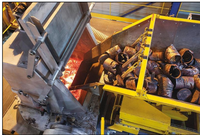
Figure 5.9. UPCAST ® , Finland apply the technology of an automatic feeding table for their upward continuous casting machines [64].
