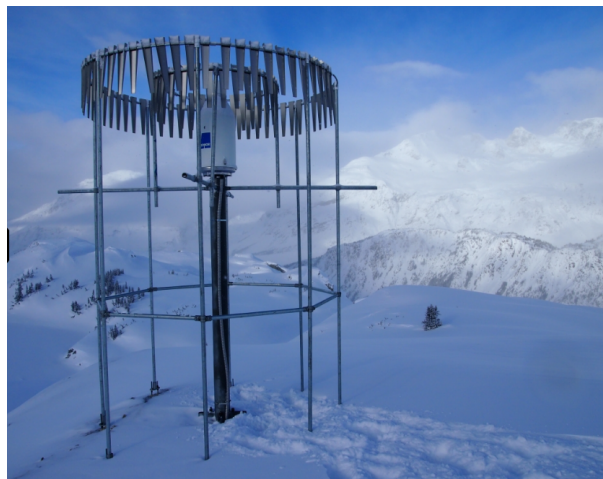
Figure 5: SMHI uses automated rain gauges of the brand Geonor. Depicted is model T-200B on a stand, along with wind shields.
