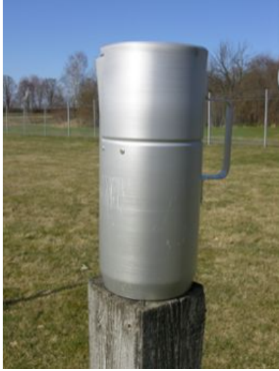
Figure 3: A rain collector, used on manual SMHI precipitation stations.
