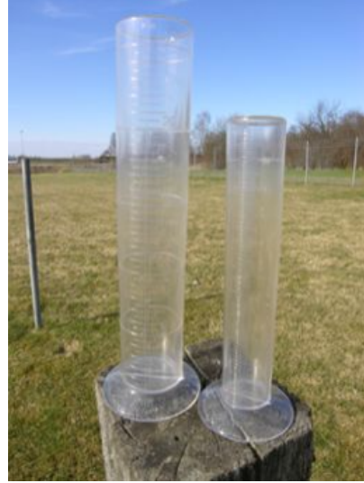
Figure 4: Collected rain is measured manually using measuring glasses.
