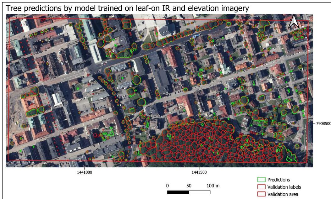
Figure 19. Validation area with tree predictions by model trained on leaf-on IR and CHM imagery.
