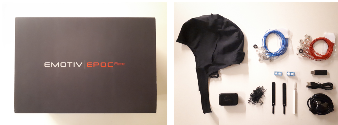
Figure A.1: Emotiv Epoc Flex gel sensor kit with 32 Ag/AgCl (silver-silver chloride) electrodes. This device has a sample rate of 128 SPS (samples per second) at a frequency range of 0.16–43 Hz. The electrodes and wires are individually thread through the cap and positioned according to the International 10-20 system. There is a control box that receives signals from the electrodes and transmits them wirelessly to a USB receiver connected to a computer.
