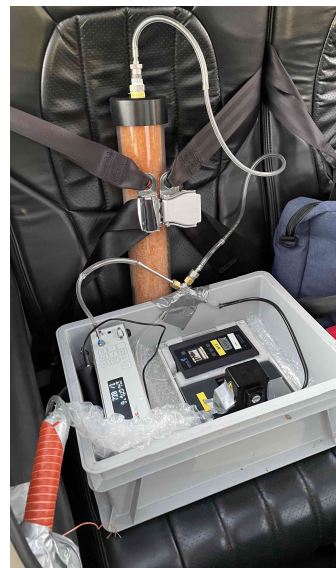
Figure A.3: Sensor set up on the back seat of the aircraft, with the common inlet to the sensors fed into the air outlet.
