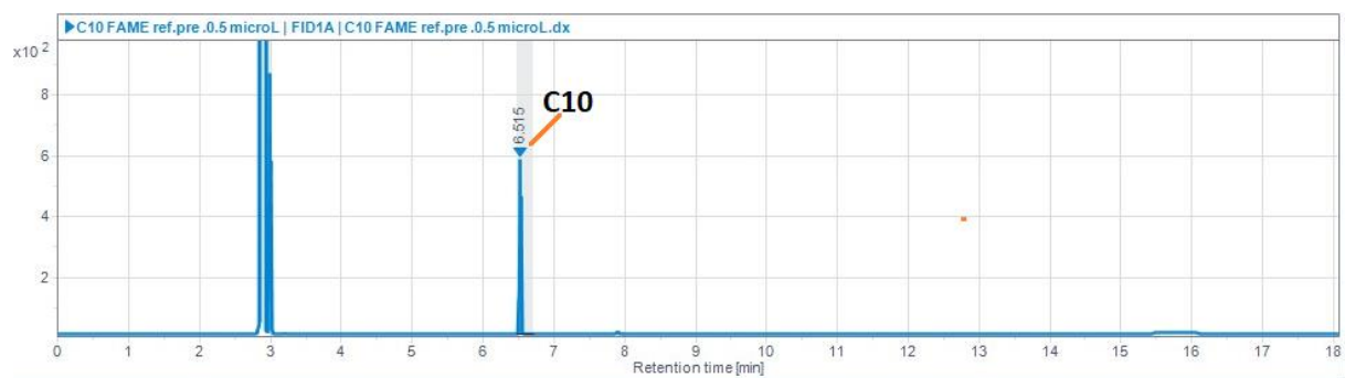
Figure 3: Chromatogram of pre-synthesized methyl decanoate, tR: 6.515.
