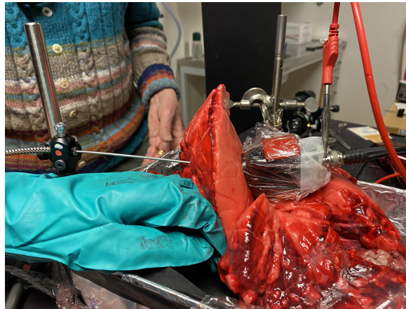
Figure 4.2: Wild boar lung filled with air with the optic fibre and detector visible, show how the transmission measurements were performed. To prevent the optic fibre from poking a hole in the lung tissue, the lungs was held in place during the measurements.
