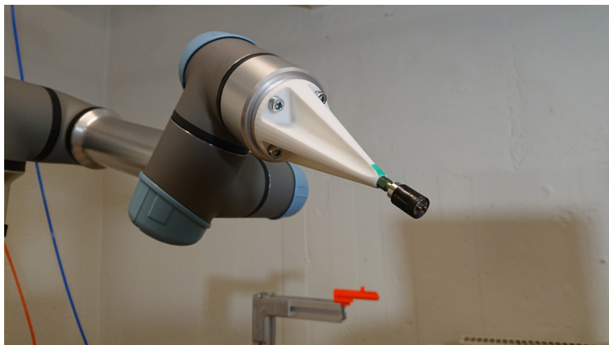
Figure 4.2 The UR5 robot with the custom tool holding the bit.
