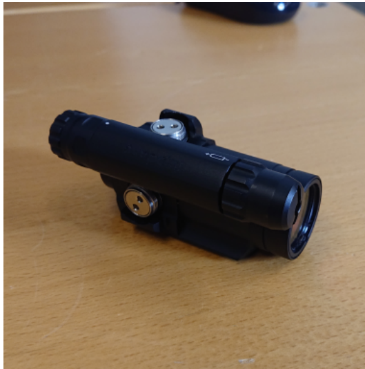
Figure 3.4 A red dot sight from Aimpoint, model compM5
