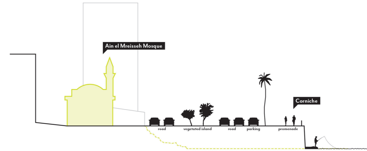
FIG. 31: Schematic section of the Corniche near the Ain el Mreisseh Mosque (based on dimensions measured in Google Earth Pro).
