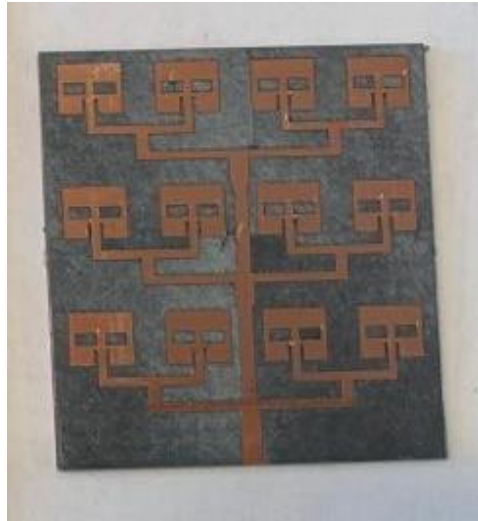
Figure 7.2: Manufactured receiver 3×4 antenna array without connector.
