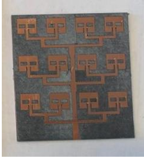
Figure 7.2: Manufactured receiver 3×4 antenna array without connector.
